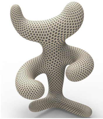
Figure 19: We show a (3, 4, 6, 4) pattern on the Moomoo model with 57 singularities. This is the most complicated model shown in the paper due to the high number of singularities (hexagons replaced by septagons and pentagons) and the high curvature variations.
