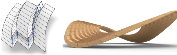
Fig. 9. Discrete principal pleated structures are conical meshes and have offsets at constant distance. Right: A wooden construction of constant thickness based on a PPLS. Observe the clean intersection of elements in the nodes which does not occur if the guiding mesh fails to be conical.
