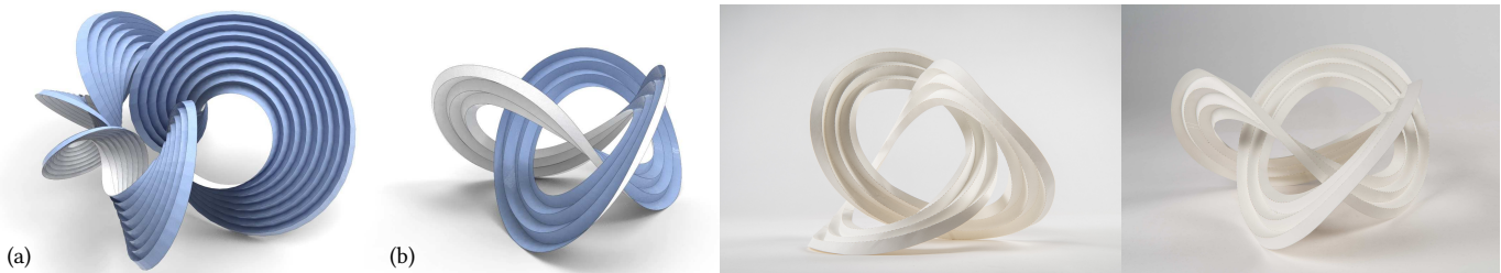
Fig. 24. Our paper is inspired by curved-folding art, and these examples in particular have been motivated by Erik and Martin Demaine’s curved-folding sculptures. The pleated structures shown here have been computed by propagating pseudo-geodesics from a space curve in the manner of Fig. 19. The paper model has been made on the basis of the development we computed as part of our optimization procedure.
