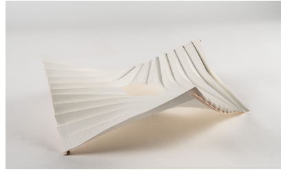
Fig. 22. By following the asymptotic curves on a negatively curved surface, we create a pleated structure with upright folding and combinatorial singularities. We show both a rendering and a photo of a paper model.
