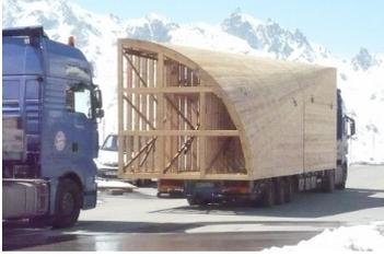
**Figure 2:** Formworks for concrete tunnel of variable cross section (Silvretta reservoir, cf. [www.spezial-schalungen.com](http://www.spezial-schalungen.com)).
