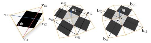
Figure 11: Geometric constraints for angles (left), planar white quads (middle) and A-nets (right).
