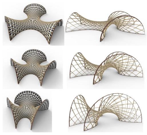
Figure 9: A-nets with constant angle  $60^\circ$  (top),  $75^\circ$  (middle) and  $90^\circ$  (bottom). They represent surfaces with constant principal curvature ratio  $\kappa_1/\kappa_2=C$  with C=-1/3 (top), C=-0.58879 (middle) and C=-1 (bottom). The latter surface is a minimal surface. Left: One diagonal mesh and the associated checkerboard pattern. Right: The diagonal mesh has been used as a basis for an asymptotic gridshell with constant node angle.
