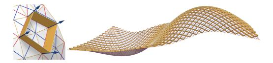
Figure 3: Principal meshes in the diagonal mesh approach have discrete surface normals which are suitable as node axes of a torsion free support structure. Left: The node axis at a vertex of one diagonal mesh (red) is orthogonal to the corresponding planar face of the other diagonal mesh (blue). Hence, node axes at connected vertices lie in the normal plane of the orthogonal crossing diagonal (blue). Right: Torsion free support structure attached to a principal diagonal mesh.
