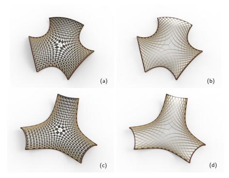
Figure 13: Angles as a design parameter. A-nets as checkerboard patterns (a,c) and asymptotic gridshells (b,d). For (a,b), the angle increases radially from the central singularity to the boundaries, in (c,d) it decreases.
