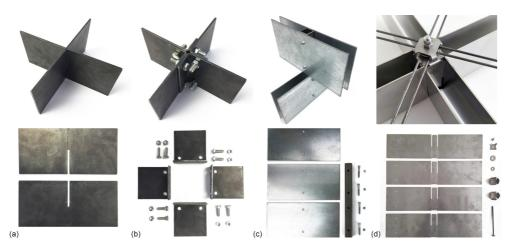
Figure 15: Development of orthogonal steel joints, looking at (a) a simple slotted and welded connection (b) segmented, reciprocal lamellas, (c) double lamellas on two levels connected by a square pipe and (d) a double slotted connection with star-shaped connectors. The latter was used for the construction of the Asymptotic Gridshell.
