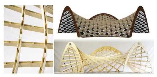
Figure 14: Diagonal mesh and associated checkerboard pattern of an A-Net with constant angle  $90^{\circ}$  on a Schwarz D minimal surface (top right). The Timber prototype is constructed with a slightly coarser network (bottom right). We introduce two parallel lamellas to allow for bending and post-coupling of the slender profiles. The two families of lamellas are constructed on separate levels and connected with square studs (left).
