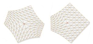
Figure 4: The angle between two diagonals can be determined by the rotation from one diagonal (black) to the other. This requires the selection of one diagonal per quad so that they form fair polylines, which is only possible for even valence v (left, v=6), but fails for odd valence (right, v=5).
