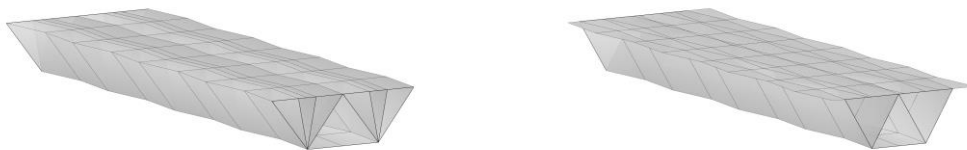
Figure 6. Concept sketch of the two bridge concepts the zipper tube (left) and the nested solution (right) in its final folded state
