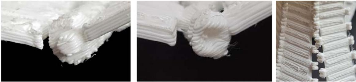
Figure 6: Detail of the still working RH-Snap element and a semi-assembled curved foldline.
